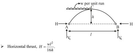
**Case VIII:** A two hinged parabolic arch of span '*l*' and rise '*h*' carrying a load varying uniformly from zero at the left end to *w* per unit run at right end. EI = constant.
