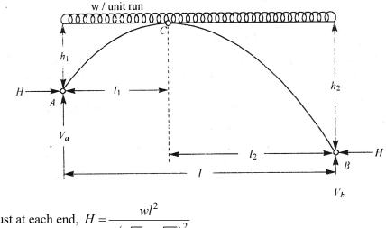
➢ Horizontal thrust at each end, H =  $\frac{wl^2}{2\left(\sqrt{h_1} + \sqrt{h_2}\right)^2}$
