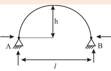
> Two hinged arch is statically indeterminate to 1 degree.
