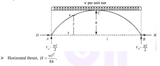
**Case VII:** A two-hinged parabolic arch carrying a u.d.l. of w per unit run on its left half of the span. EI = constant
