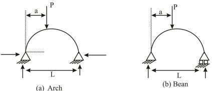
In the above example, figure (b) is not an arch, as there is no horizontal reaction is developed.
