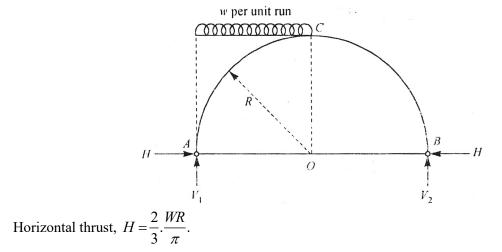
**Case V:** A two-hinged semicircular arch of radius R carrying a distributed load uniformly varying from zero at the left end to w per unit run at the right end. EI = constant
